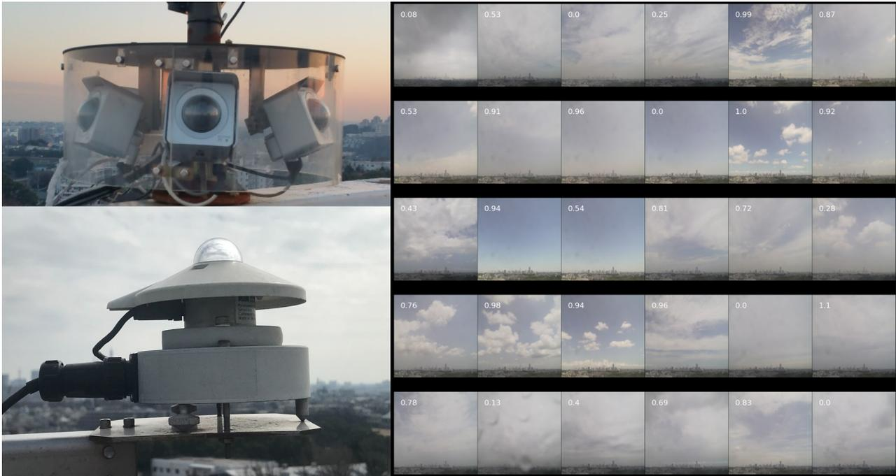
Fig. 1. Left: Camera and pyranometer installed on the roof of Yokohama National University. Images and solar radiation are measured every minute. Five cameras cover directions of Mt. Fuji (west), Machida (northwest), Tokyo (northeast), Minatomirai (southeast), and Kamakura (south). Right: Camera images (southeast direction) at 12:00 AM in July 2017, arranged for 30 days. The number in the upper left of each image shows the solar radiation in  $\text{kW/m}^2$ .
